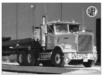
Thurman's 8560 Series is a low profile, electronic truck scale built to provide many years of rugged, dependable truck weighing.
