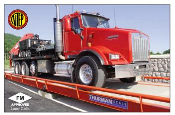
Thurman's DiamondBack Field Pour Truck Scales feature a 10" thick concrete deck for maximum strength and a unique "sealed deck" design that protects the scale's structural steel supports from moisture intrusion.
